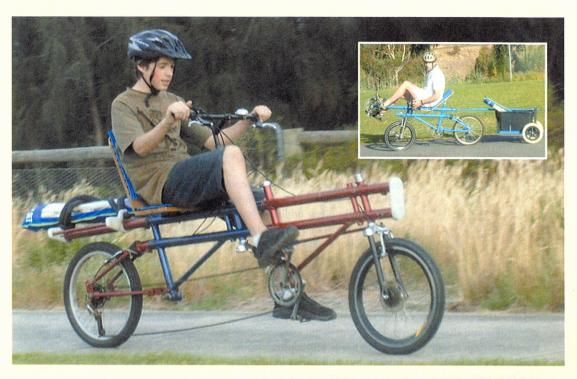
rack, trailer and recumbent seat & boom. The frame has attachment points at the ends for holding another frame or extras, a tube that acts as a static handlebar mount, and tubes that can support pulleys for a front-wheel drive mechanism. The seatpost doubles as a mount for the recumbent seat, as do the bottle mount bosses on the top tubes. I have taken care to ensure that the extra features on the bike don't look scrappy when unused – for example a plastic plate can fit
